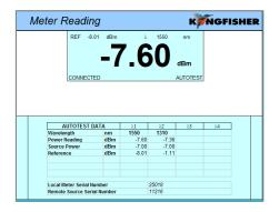
Live Data Sheet is for cable acceptance testing and instant pass / marginal / fail analysis at up to 4 wavelengths. Its main functions are on-site test configuration and acquisition. Project & instrument related information is also stored with the testing data. The sheet is auto-setup for 1 or 2 directional test during Autotest. In data Secure Mode, data is protected against unauthorized modification.
