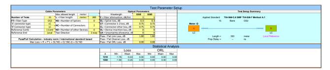
**Final Report Sheet** is a default reporting sheet which also provides backwards compatibility with report formats in KITS™ version 3.02 or earlier, and is suitable for typical 2 wavelengths testing.
