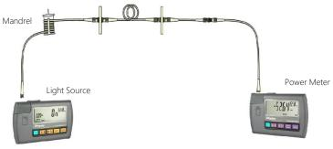
Figure: Test the multimode fiber link accurately using Kingfisher's Multimode Mandrel
