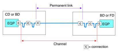
Figure 3, Link - channel definition
