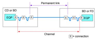
Figure 4, Link - channel definition
