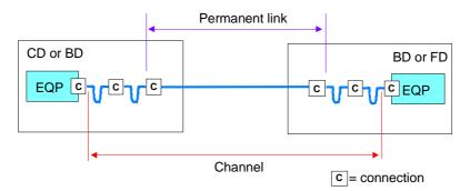
Figure 4, Link - channel definition
