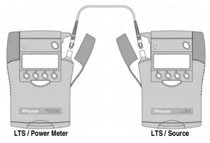
Test set-up for both the Output Power and Short Term Stability Tests
