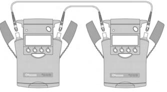
Simultaneous one way loss testing
