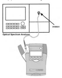
Test set-up for the centre  $\lambda$  and spectral bandwidth
