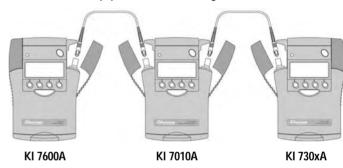
Test set-up for the Power Meter Accuracy Test
