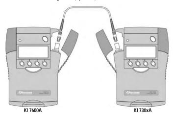
Test set-up for the Short Term Stability Test
