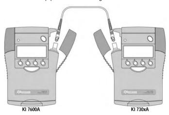
Test set-up for the Output Power Test
