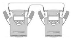
Put each instrument into Autotest before connecting the patch-leads. Note the results will be stored on both instruments and then merged later, so records management needs extra care.
