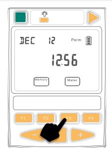
2 Press [Toggle centre]: The current ID tag in used will be displayed and flashing.
