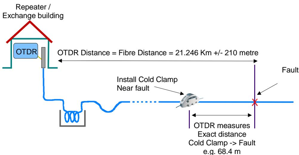
The Cold Clamp system has been proven on cables containing acrylate coated optical fibre with jelly filling (it may also work on other cable types). It can be used on optical fibre cables carrying live traffic, and on armoured cable. On armoured cable, a high nitrogen boil off rate occurs due to heat conduction along the armouring.
