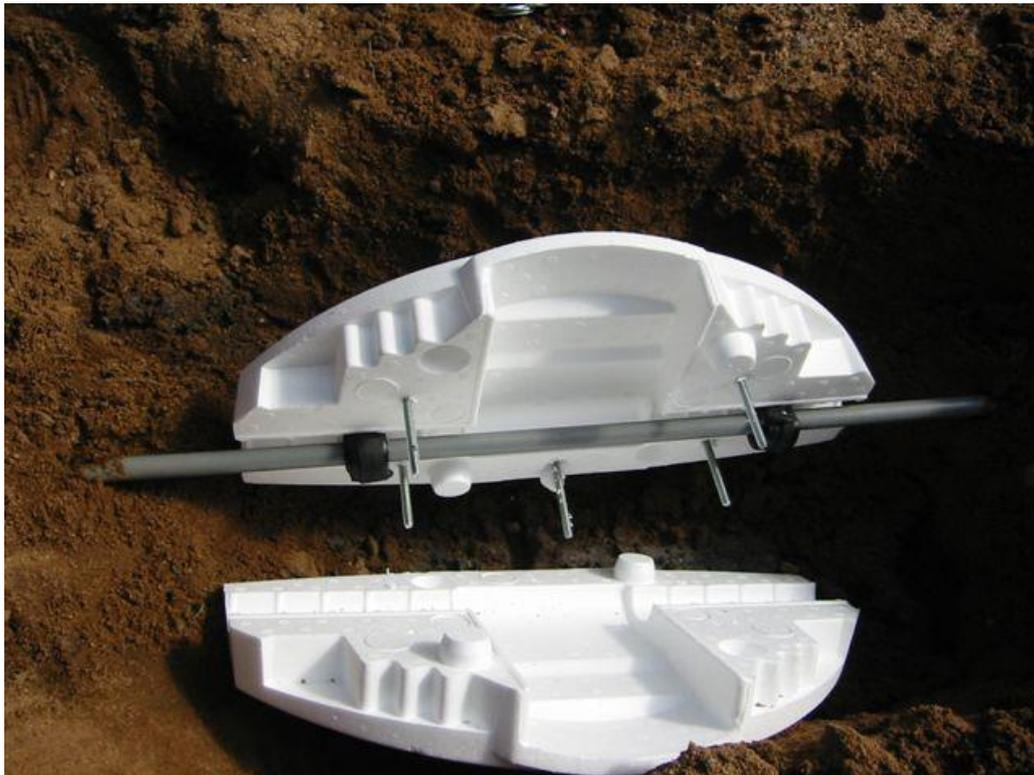
Position the two halves of the Cold Clamp reservoir together with the top facing up and the seals positioned in the glands. Place the threaded rods, washers and wing nuts and tighten the wing nuts in sequence, bringing the foam halves firmly together to create a good seal around the liquid nitrogen chamber.
