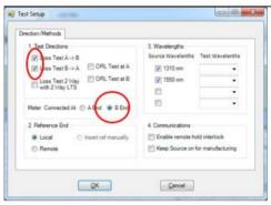
2 Select the 1'st 2'nd locations of memory in instrument to download: Select command, [Memory Download]. Enter "1" for "Start Memory", "2" for "No. of Fibers" and "1" for "Start at Fiber No" as below.
