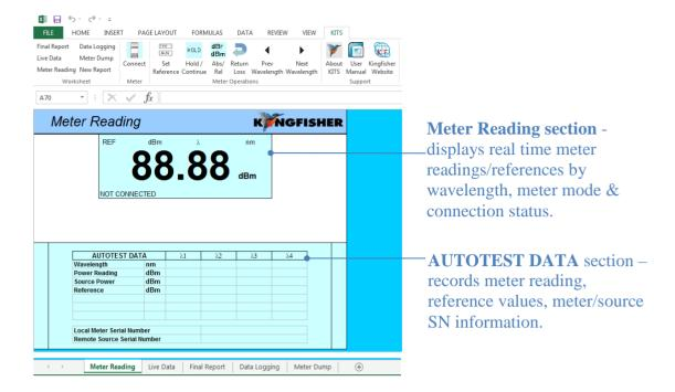
The "**Meter Reading**" work sheet provides basic meter functions and is useful for confirming instrument connection, and where a large display is required. This worksheet is opened by default when KITS<sup>TM</sup> completes start-up.
