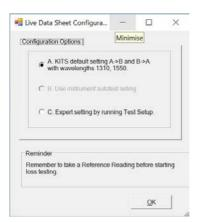
Click "OK" to proceed will result in Test Result section of the opened worksheet automatically configured with the wavelengths 1310, 1550 nm.
