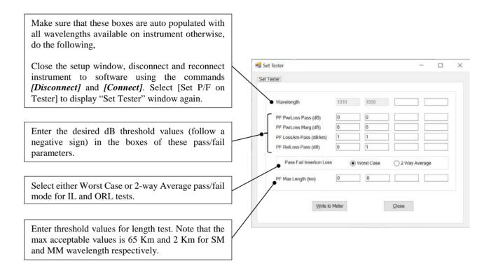
Click on "Write to Meter" button to save the entered values and selection on the Set Tester window to the connected instrument. When prompted with the popup box below, click "OK" to proceed.
