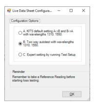
Click "OK" now will result in Test Result section of the open worksheet automatically configured with all active wavelengths (1310, 1550 nm in this example).
