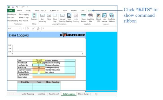
The Data Logging sheet supports data logging whether the meter is in Power Meter, one-way or two-way Autotest mode.
